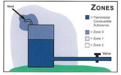
Zone 0 and Zone 20 - Permanent presence of explosive atmosphere. Only specially designed electric motors can be used here.
